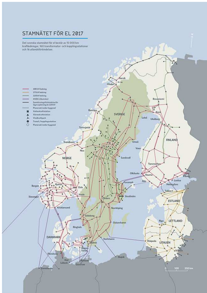
Figure 53. The grid, connectors and interconnectors in the Nordic area (existing and planned). Source: Svenska Kraftnät; Stamnätet 2017; https://www.svk.se/drift-av-stamnätet/stamnätetskartor/
