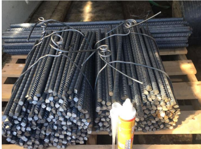
BARRAS ACERO 700 \Phi 16mm L = 0,6- 1,0 m
