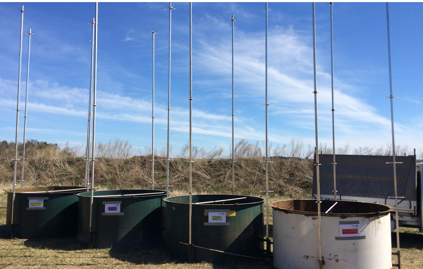
Experimental set up with containers and masts for ammonia measurements with passive flux samplers. Photo: Lena Rodhe, RISE
