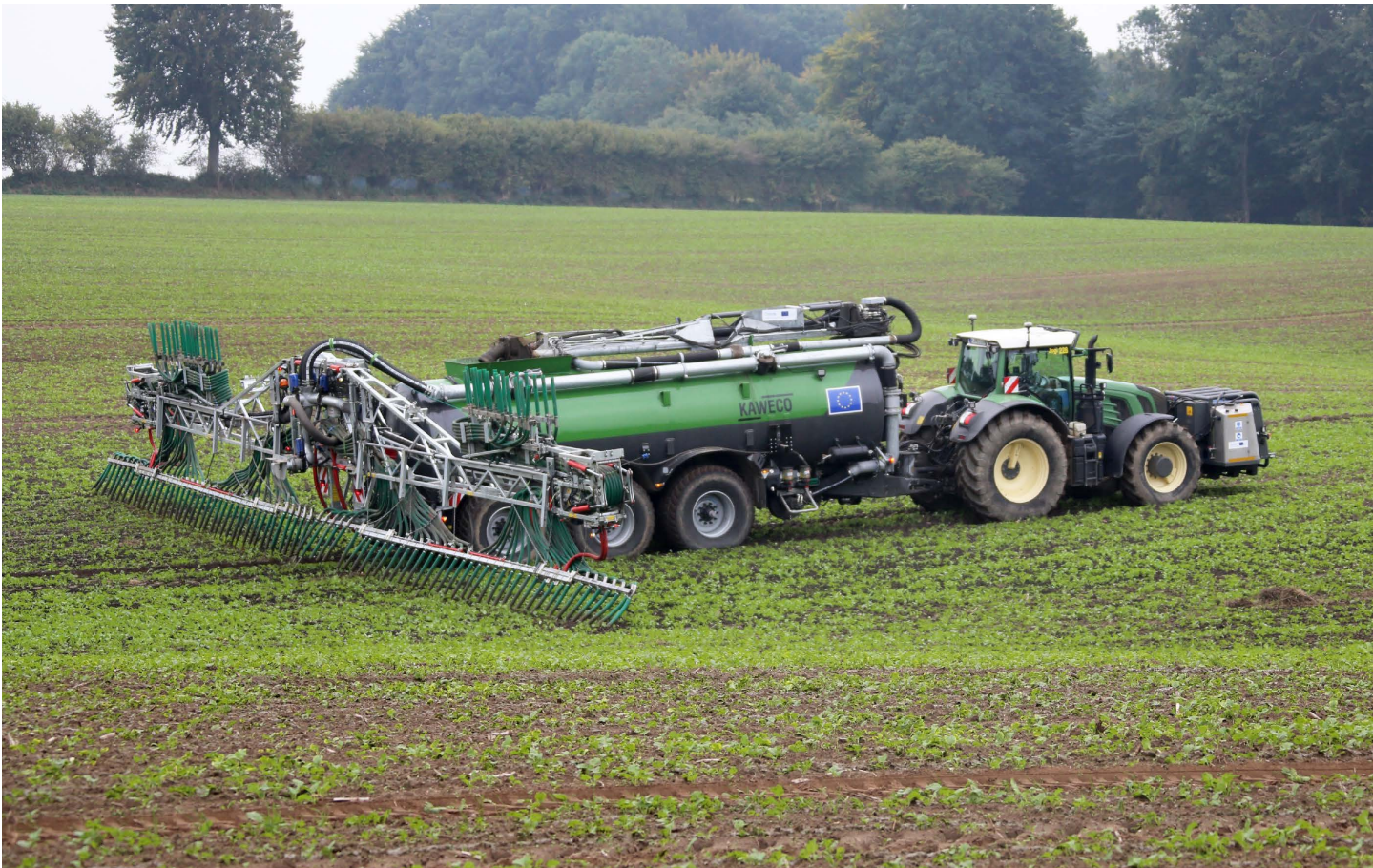
In-field slurry spreader with acid tank in Germany. Photo: Frank Steinmann, LLUR
