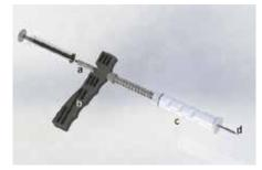
Figure 5: CAD model of the injection device developed with connector (a), ergonomic handle (b), depth limiter (c) and cannula (d).
