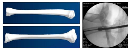
Figure 4: Sample sheep bones from additive manufacturing (left) and X-ray image from a sheep cadlab with master scale for dimension reference.
