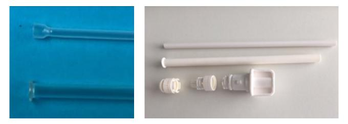
Figure 2:The extruded cannulas for the BONEBANK harvesting device. The tubes (inner and outer cannula) are manufactured from polypropylene (PP) and temperature-formed at their ends (see left) to allow glue-free assembly with the cannula adapter parts (shown on the right).
