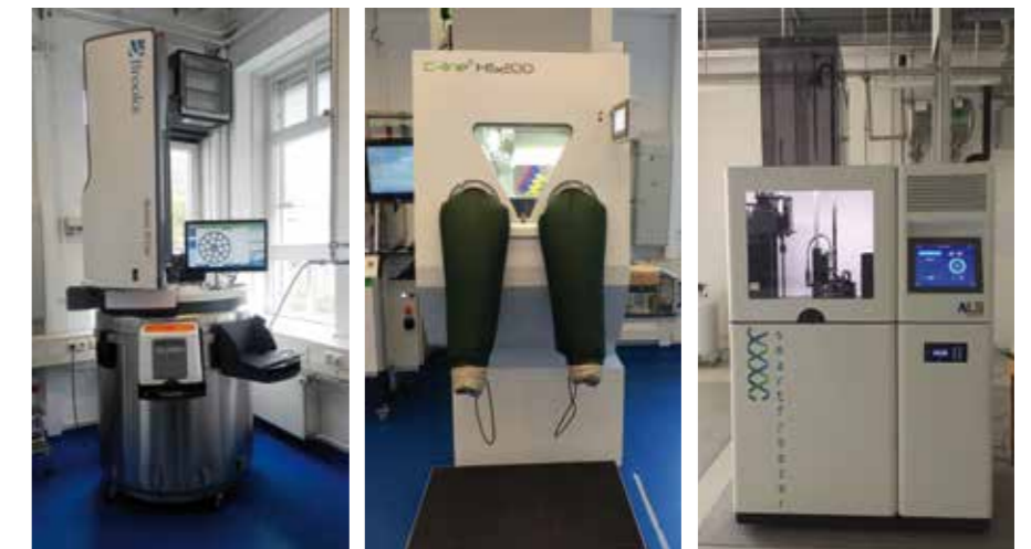
(semi-) automated nitrogen tanks: BioStore (TM) III 1500 Cryo (Brooks Automation Inc.), C-line® HS200 S (Askion GmbH), Smartfreezer® VI 80-20 (Sysmex Suisse AG)
