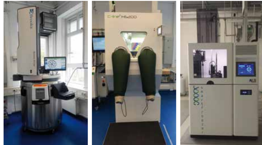
(semi-) automated nitrogen tanks: BioStore (TM) III 1500 Cryo (Brooks Automation Inc.), C-line® HS200 S (Askion GmbH), Smartfreezer® V180-20 (Sysmex Suisse AG)
