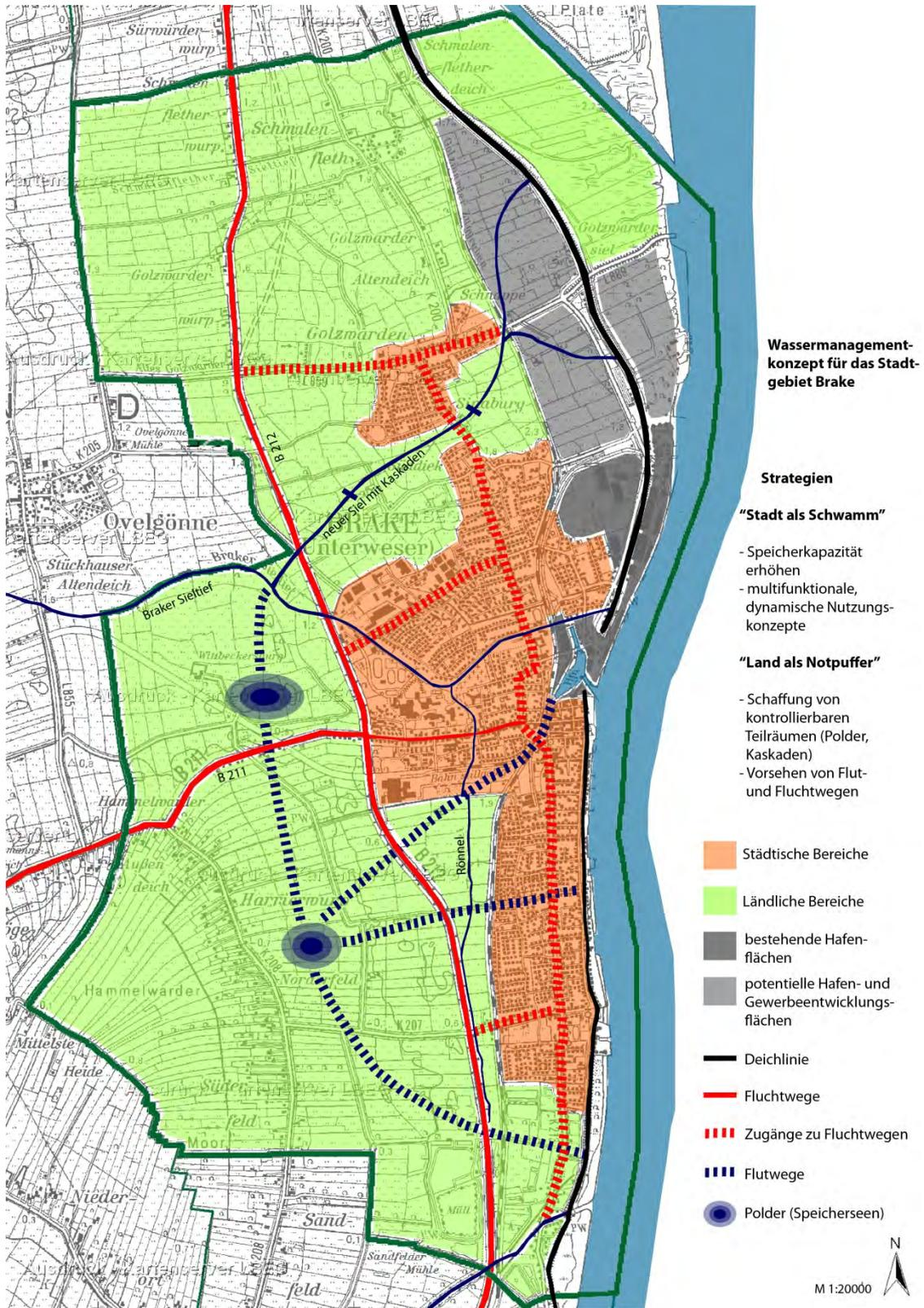
Figure 17: Draft of the urban drainage solution options within the EU Interreg IVB project CPA (in German).
