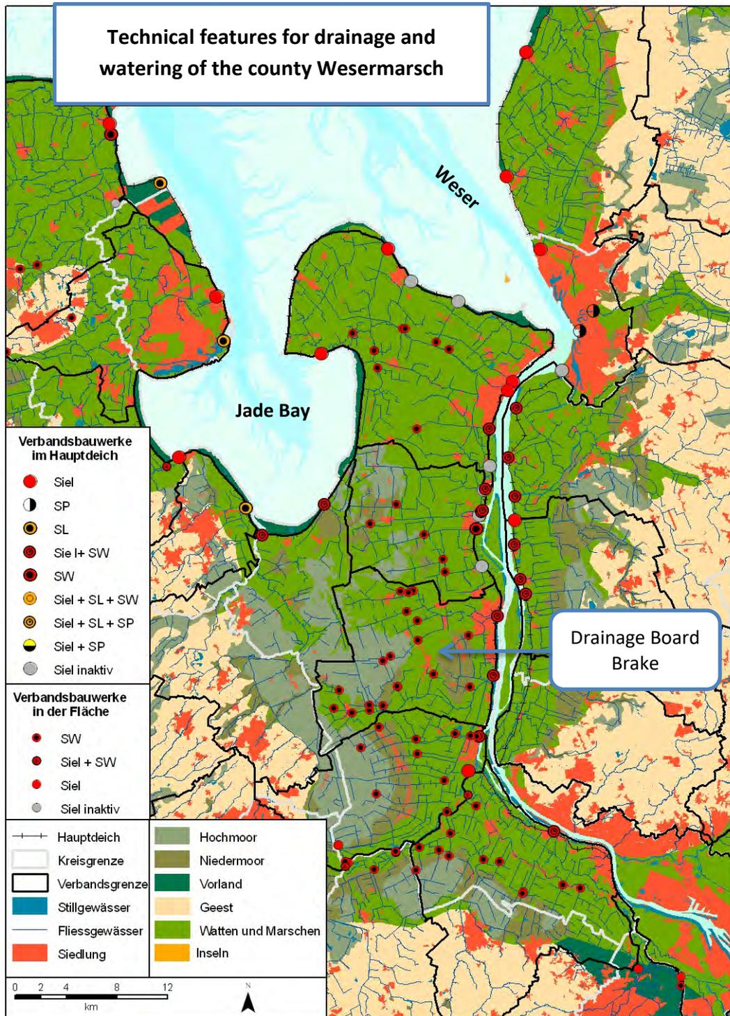
Figure 6: This map shows the water boards and the technical features to ensure the drainage and watering of the northern part of the county Wesermarsch. Source: modified after Ahlhorn et al. (2010)
