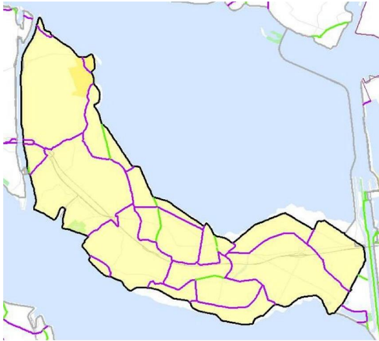
Figure 3.2 Inner dykes within dyke ring 31. Purple: inner dyke with water management function, green: inner dyke without water management function (source: VNK2 report 'Flood risk Dike ring 31 Zuid-Beveland', December 2011)
