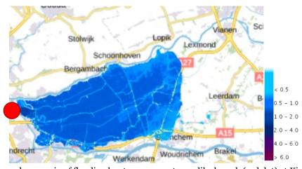
*Figure 3.3* Example scenario of flooding by storm surge at sea, dike breach (red dot) at Kinderdijk (source: LIWO)
