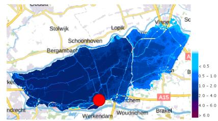
*Figure 3.1* Example river flooding scenario, dike breach (red dot) at Hardinxveld-Giessendam east (source: LIWO)
