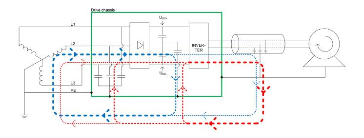
"Red" currents relate to inverter switch frequency and harmonics, >10MHz "Blue" currents relate to grid frequency: 50Hz and harmonics
