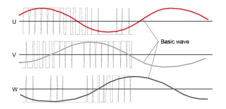
PWM signal direct to machine is still the most common approach due to price and space advantages
