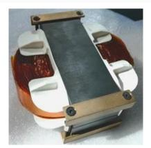
Fig. 3.2. Hardware prototype fo the 20 kW, 100 kHz transformer
