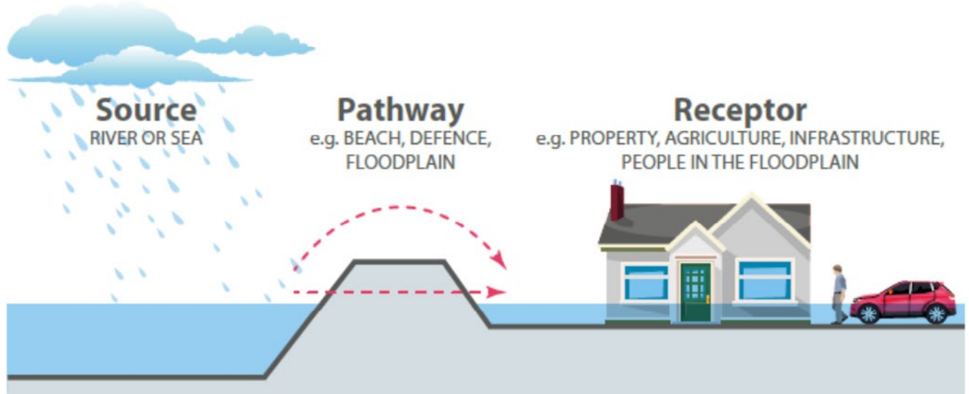
The Source-Pathway-Receptor (SPR) framework (Redrawn from Sayers et al, 2002) 4
