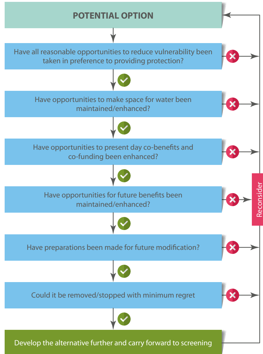
Figure 4.4 flow chart to help guide the development of adaptive management measures (Sayers et al., 2015)
