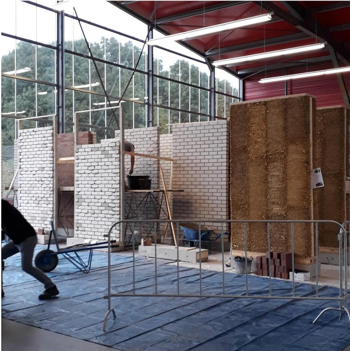
Picture 3. TNO is testing different wall elements made by fully recycled materials. (Picture by Virpi Palomäki, CE Wood -project).
