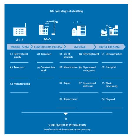
Figure 1. Building's life cycle phases (Ministry of the Environment, 2019, p.14).
