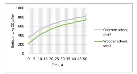
*Figure 5. Carbon footprint as a function of time: small concrete school and small wooden school.*
