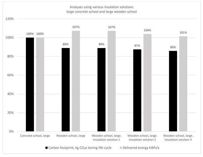
Figure 11, Analyses with various insulation solutions 1–3, large concrete school and large wooden school
