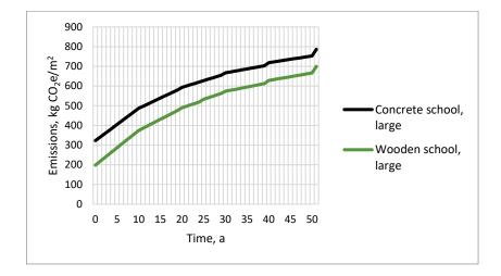
Figure 9. Carbon footprint as a function of time: large concrete school and large wooden school
