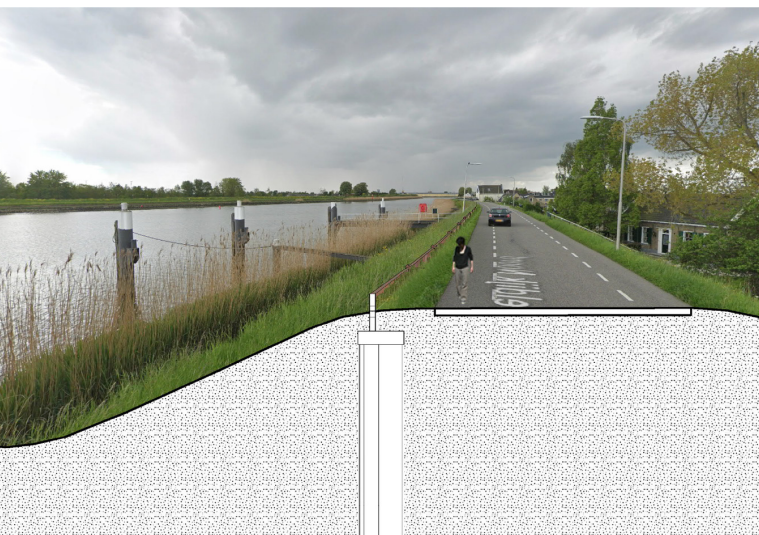
Figure 5: Adaptable design of the dike for the top of the construction. Courtesy Bosch Slabbers Landschapsarchitecten.
