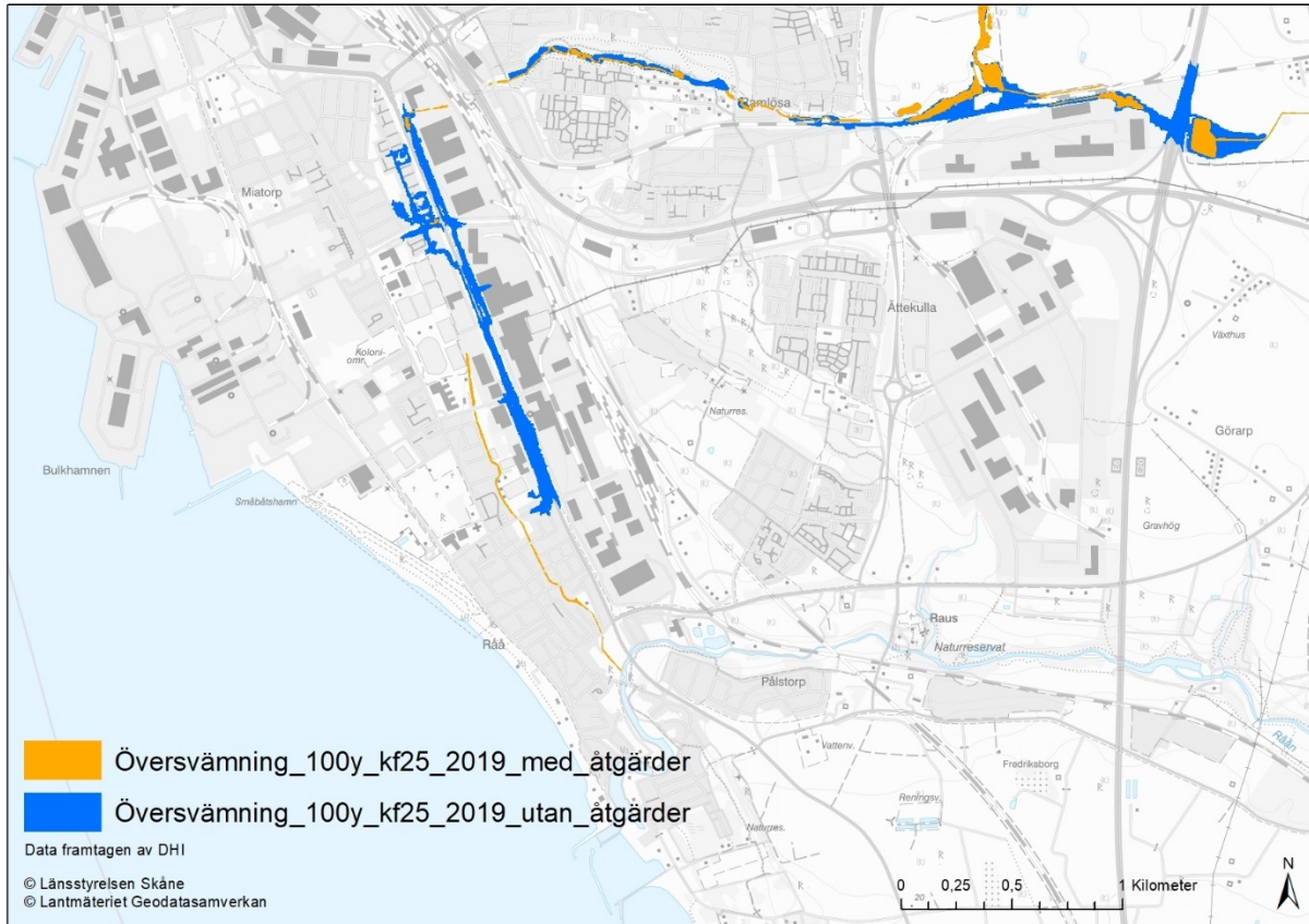
Figure 2.3.6. Flooded areas in the lower part of catchment Lussebäcken. The map shows flooded areas with measures (yellow) and without measures (blue) indicating that water is distributed in connection with measures upstream avoiding flooding downstream.
