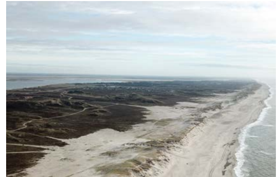
Figure 2-2: Drone image from March 28 2019. A large deposit of aeolian transported sediment is visible in the area leeward of the dune crest.
