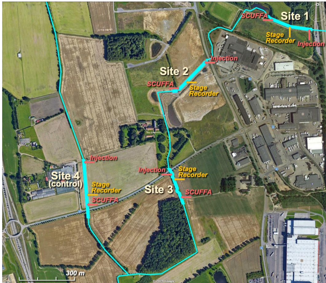
Figure 1 Map showing the relative locations of the four Lussebäcken study-sites, with positions of the automatic stage recorders and the Rhodamine WT injection & SCUFFA sites.
