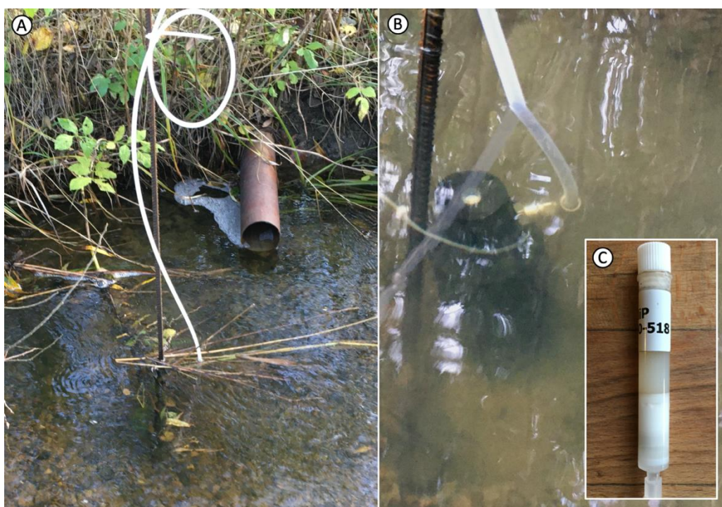
Figure 12 SorbiCell deployment: A) anchoring ca. 15 cm in the channel bed; B) WW-50 surface water sampler with static hose allowing air to exit as water is collected; C) SorbiCell NIP for PO 4 -P and NO 3 -N cartridge. Photos: EA International (October 2019).
