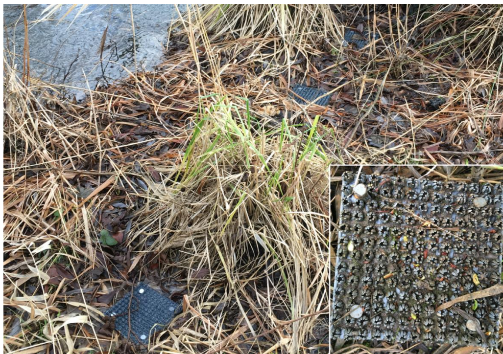
Figure 7 Set of 5 sediment traps deployed on Site 3 two-stage channel right floodplain. Photo in excerpt shows a trap at the time of retrieval. Photos: EA International (2019).
