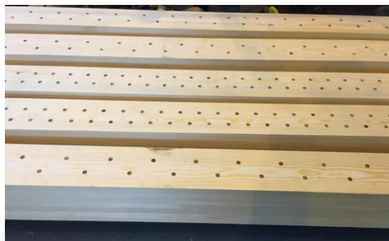
Fig. 3 - AF dowelled-laminated beams [U Liverpool].
