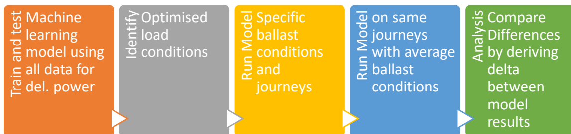
Figure 10: Approach for optimised ballast conditions analysis and savings
