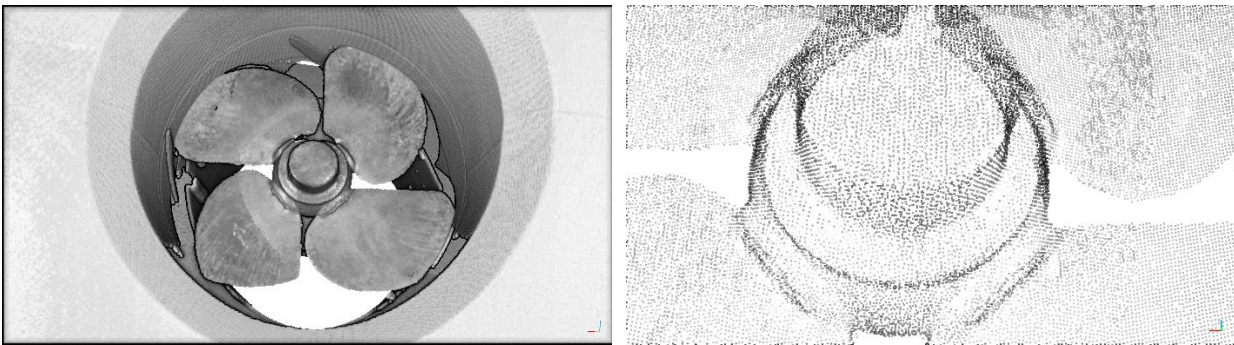
Figure 4 Rendering of point cloud data of a bow thruster captured using a 3D laser scanner: (left) viewed from a distance and (right) close up to show individual surface measurement points
