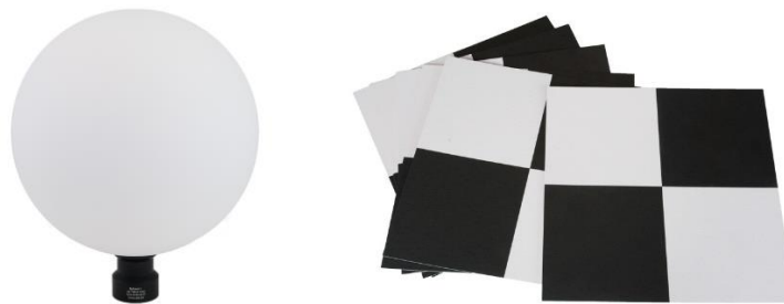
Figure 3 Artificial reference targets used when 3D scanning: (left) Spherical target and (right) Checkerboard targets
