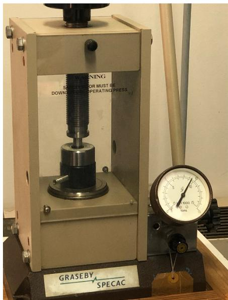
**Figure 11. Pressure machine to make the tablets**
