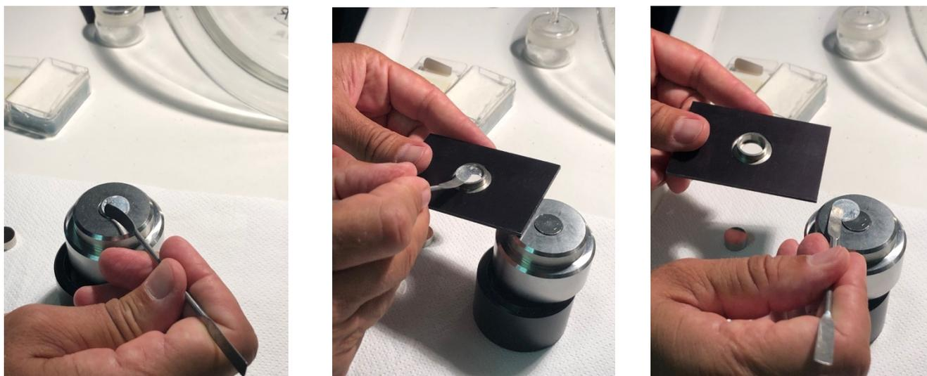
**Figure 12. Tablet obtained and inserted in the reader for the spectroscope**
