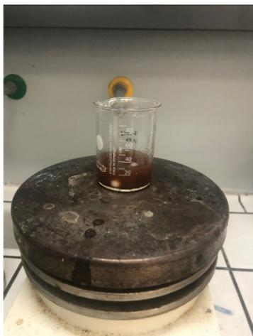
**Figure 7. Deacetylation phase using NaOH 50% solution in ratio 1:15 with sample.**
