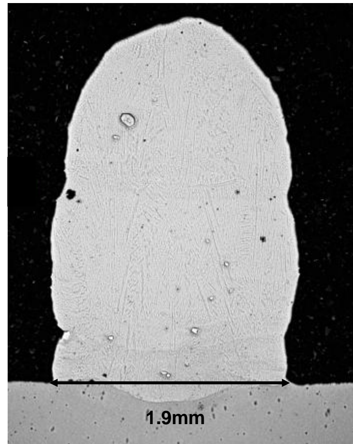
Stellite 12 ( \sim 550\text{HV}_1 ) Ø1.2mm, WFR 1.0m/min, stringer Crack-free
