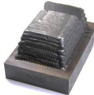
Maraging 250 steel test block on H13
