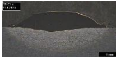
Typical shape of single-bead laser-powder cladding (Inconel 625)
