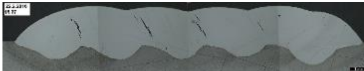
Overlay welding with CMT. martensitic steel. Cross section. Excessive penetration (~1 mm) and dilution – poor properties, hot cracking. Thickness ~2 mm.
