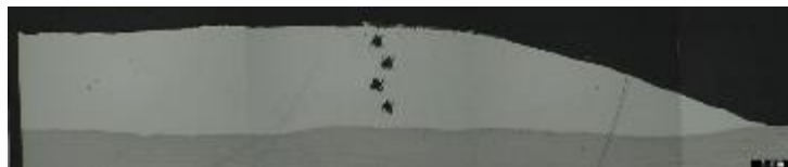
Last bead. Cross section. Low penetration and dilution Hardness 224 HV 5 .
