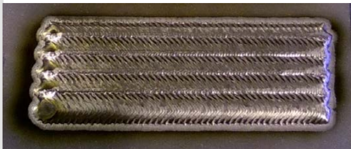
Inconel 625 test cladding with adjacent beads.
