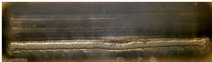
Pulsed MAG mode. Matrix hardness: 442 HV1.
