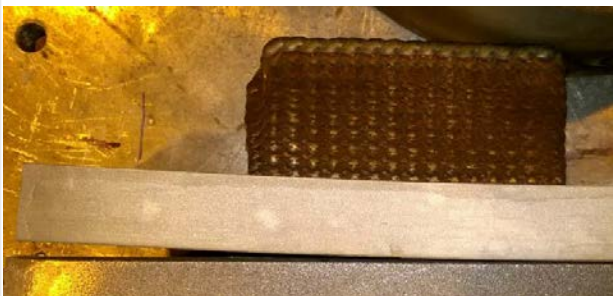
Distortion due to residual stresses
