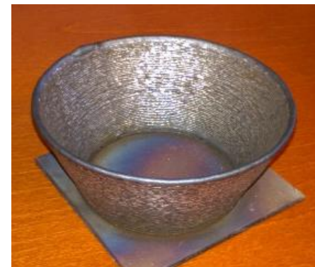
Bowl, deposition rate: 0,4 kg/h
