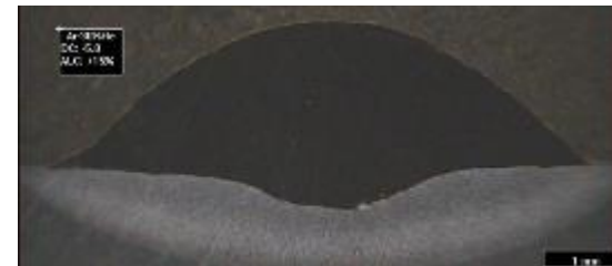
Typical shape of single-bead CMT (wire) cladding. (Inconel 625)
