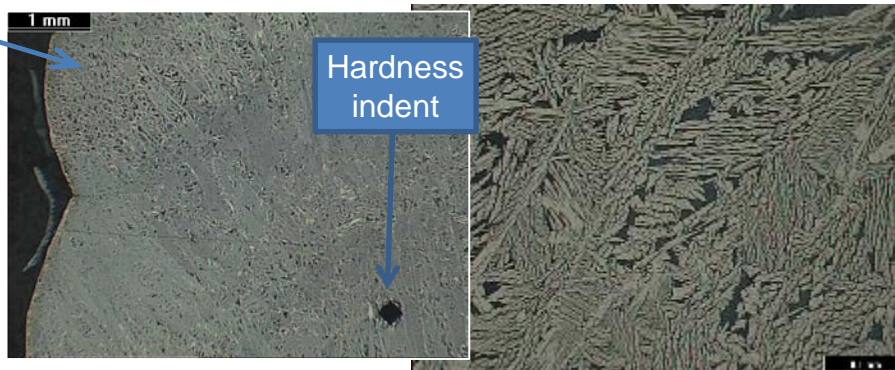
Upper part. Hardness: 240 HV 10 , austenite content: 58%
