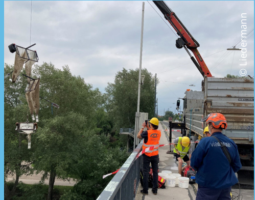
Measurement of plastic transport with specific nets on the Freudenauer harbour bridge.
