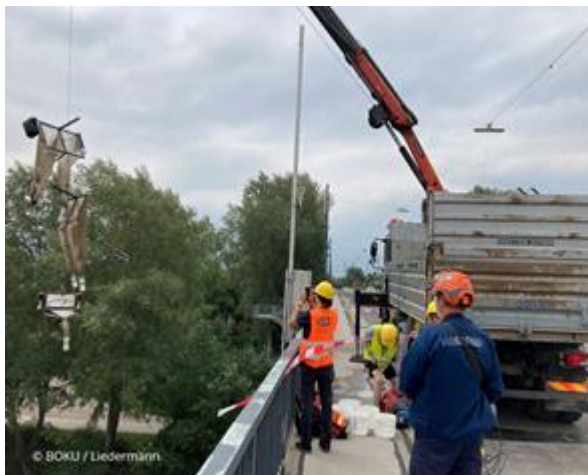
Measuring of plastic transport with nets at the Freudenau harbour bridge
