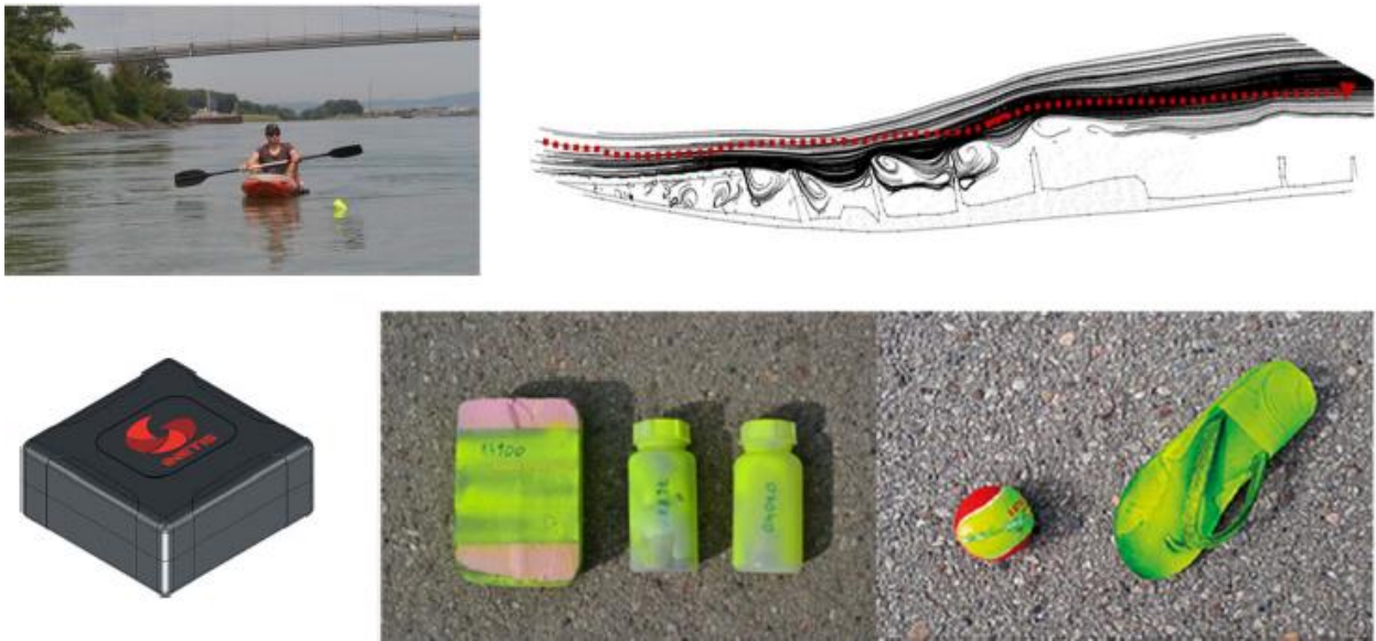
Figure 19: GPS tracking experiments to assess and validate transport, accumulation and remobilisation behaviour
