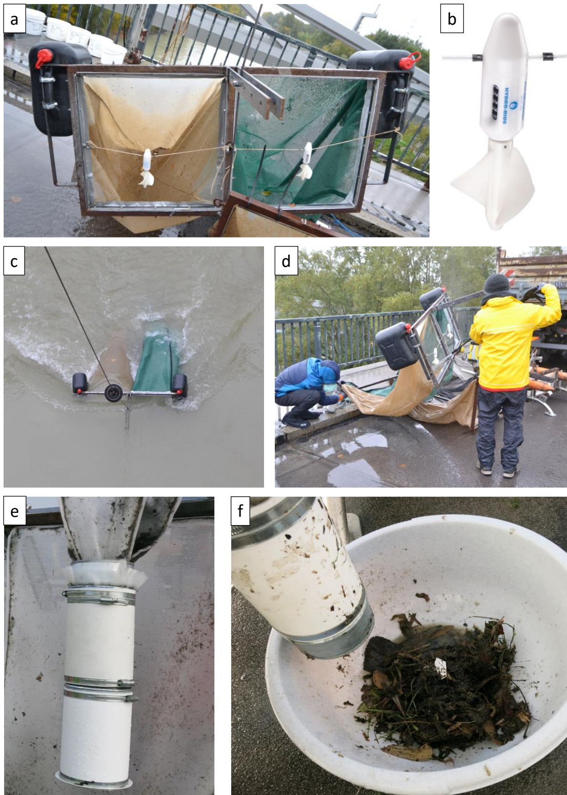
Figure 8 (a) position of the mechanical flow meters, (b) mechanical flow meter, (c) deployed device during measurement, (d) cleaning of the nets after measurement, (e) sampling container, (f) emptying a sample from the sampling container
