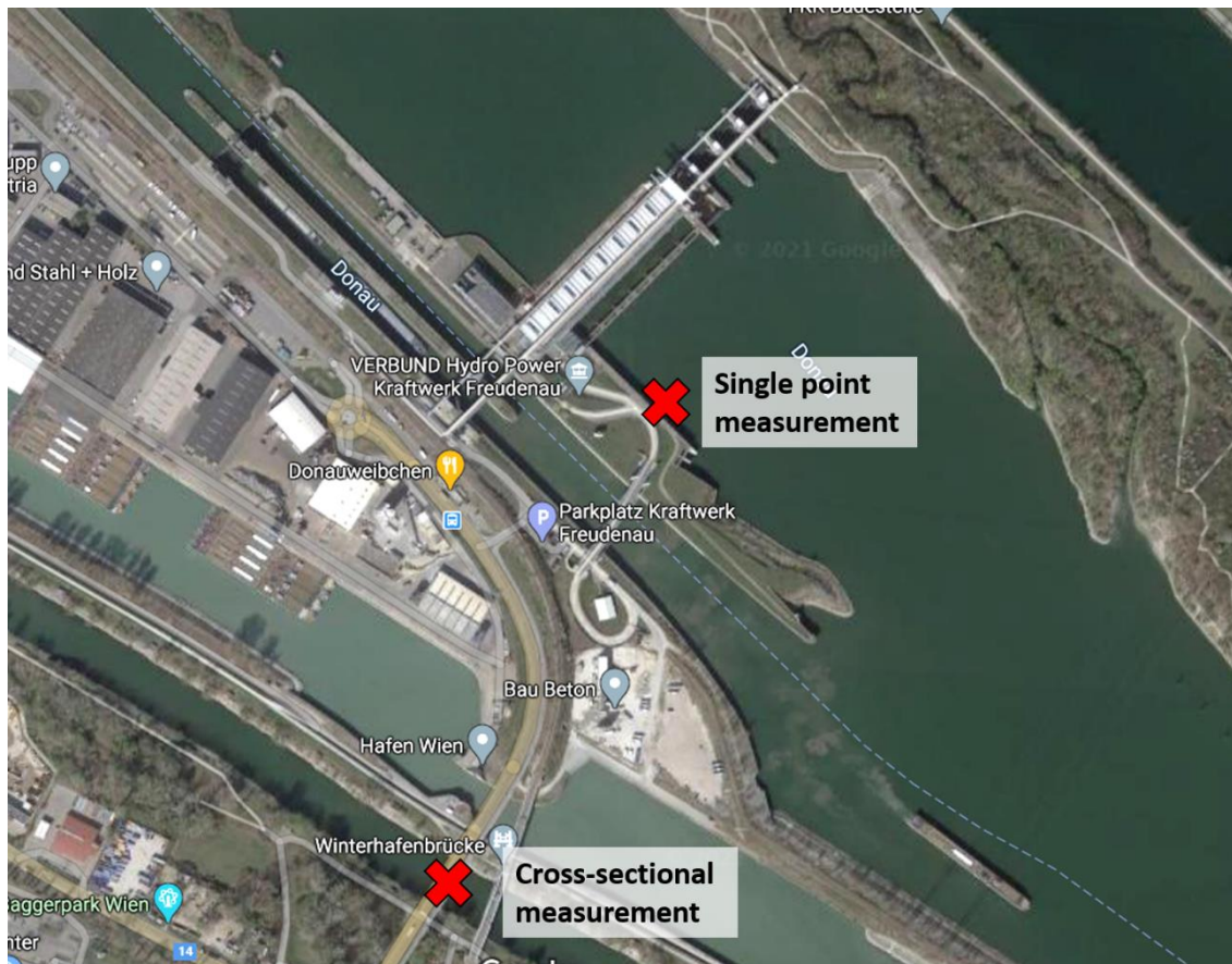
Figure 3 Locations for test measurements in order to develop a measurements device for macro plastic measurements - Single point measurements: downstream of the HPP Freudenuau - cross-sectional measurement: Donaukanal at Freudenuauer Hafenbrücke
