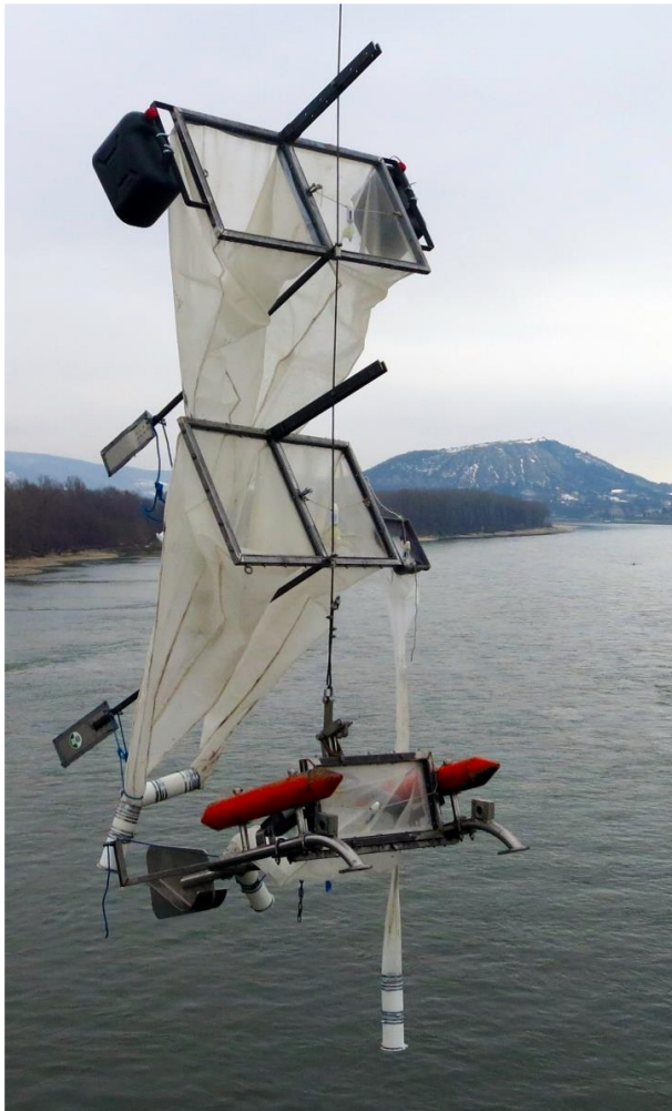
Figure 7 left: measurement device used by Liedermann et al. (2018) and right: newly developed device for macro plastic measurements within the project PlasticFreeDanube
