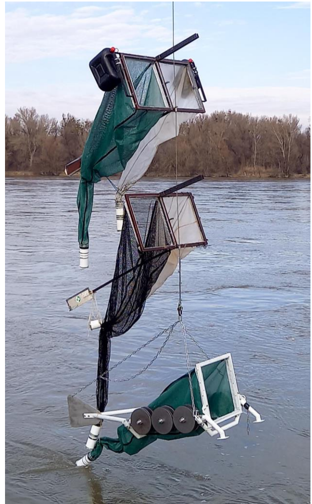
Figure 7 left: measurement device used by Liedermann et al. (2018) and right: newly developed device for macro plastic measurements within the project PlasticFreeDanube
