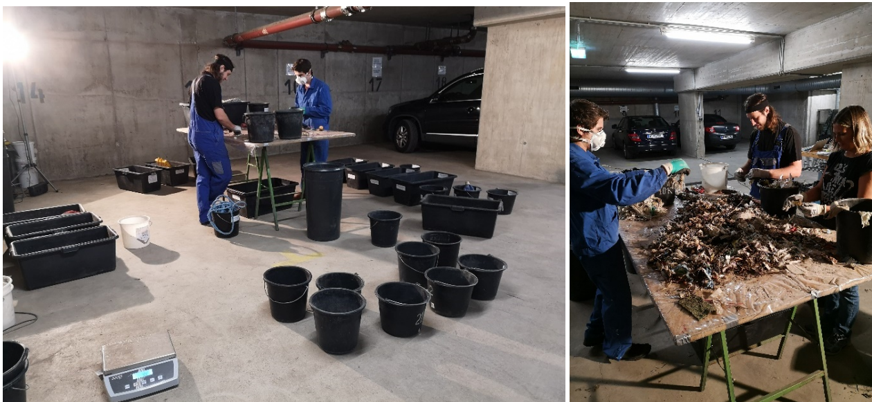
Figure: Sorting table and sorting containers for various categories
