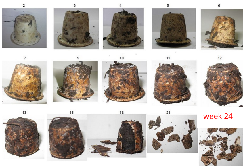
Figure 2. Temporal changes of PLA based coffee caps during 24-weeks lasting lab-scale composting experiment
