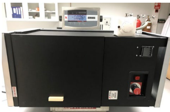
Figure 2. Modified small-scale convective dryer from Orakas Tuotteet.
