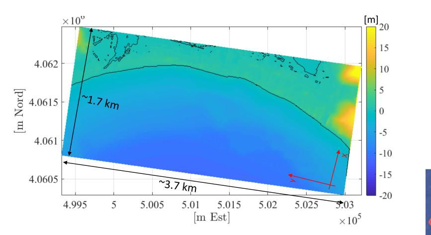
Rectilinear grid containing 207940 cells
