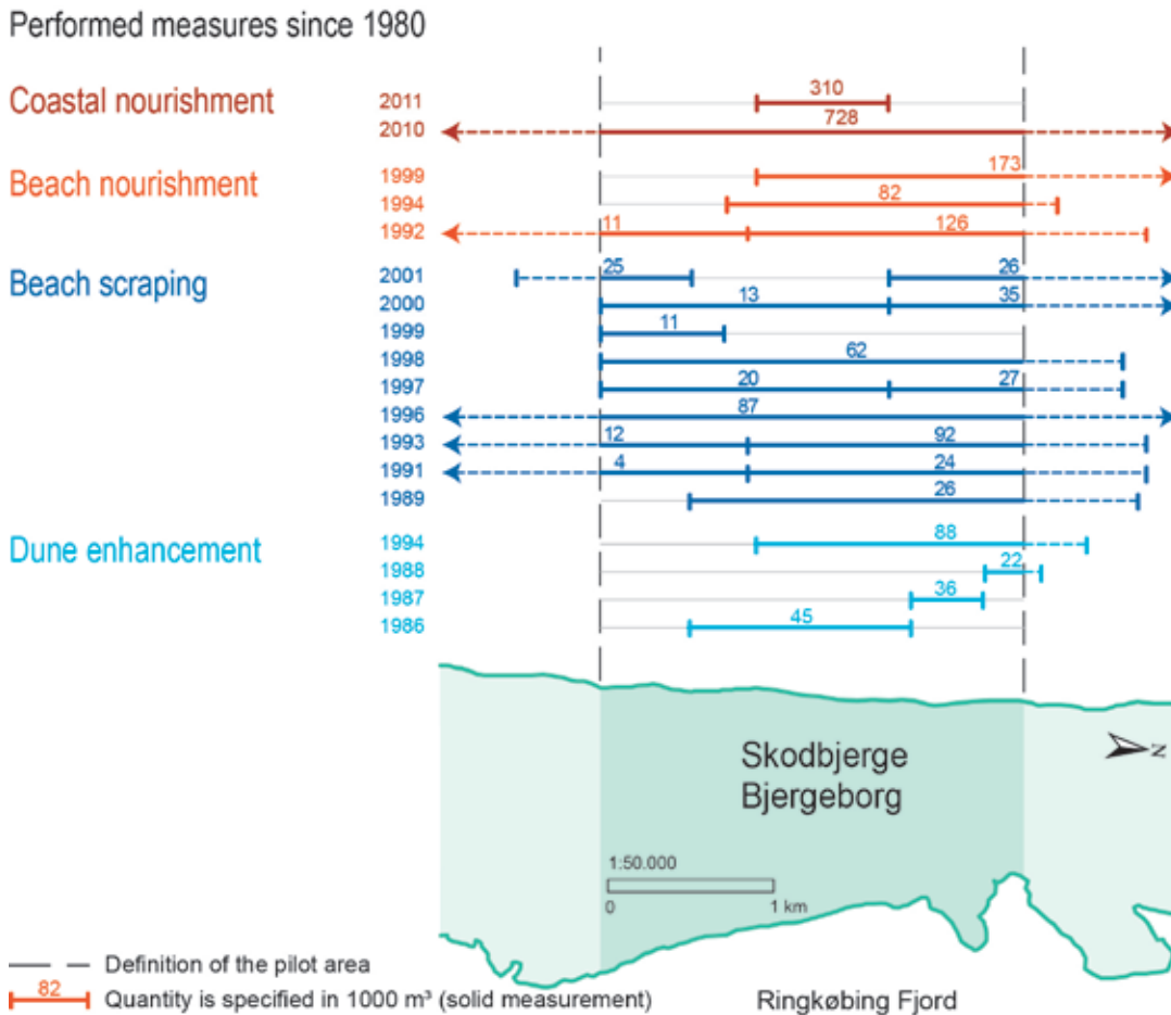
Figure 3.1 Types of coastal protection carried out in the area of Skodbjerge since 1980
