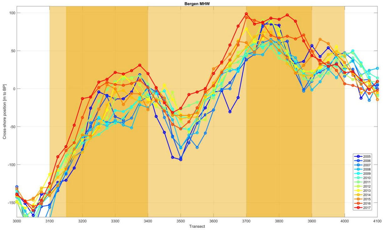
Figure 48: Position of the mean high water line for the transects in the study area (3000 is in the north, 4100 in the south) from 2005 to 2017. Squares indicate nourishment positions: shoreface nourishment (yellow) and two parts of the beach nourishment (orange).
