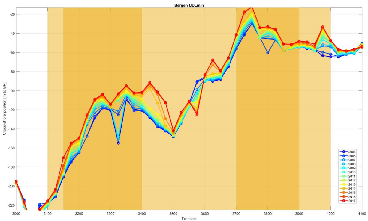
Figure 45: Position of the upper dune level for the transects in the study area (3000 is in the north, 4100 in the south) from 2005 to 2017. Squares indicate nourishment positions: shoreface nourishment (yellow) and two parts of the beach nourishment (orange).
