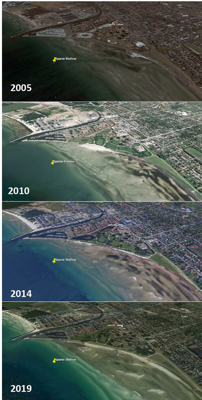
Figure 11. Evolution of Lomma beach between 2005 to 2019. The beach located in the south of the port of Lomma is nourished with sand. The sand seems to shift locations during storm events and could potentially affect the meadow and shallow limit of eelgrass which is located today at about 300m from the beach. Images from Google Earth Pro.
