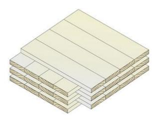
18 meters in length and 3 meters in width. The finished pre-cut CLT panels are mostly delivered directly to the construction site and can be set up very quickly.
