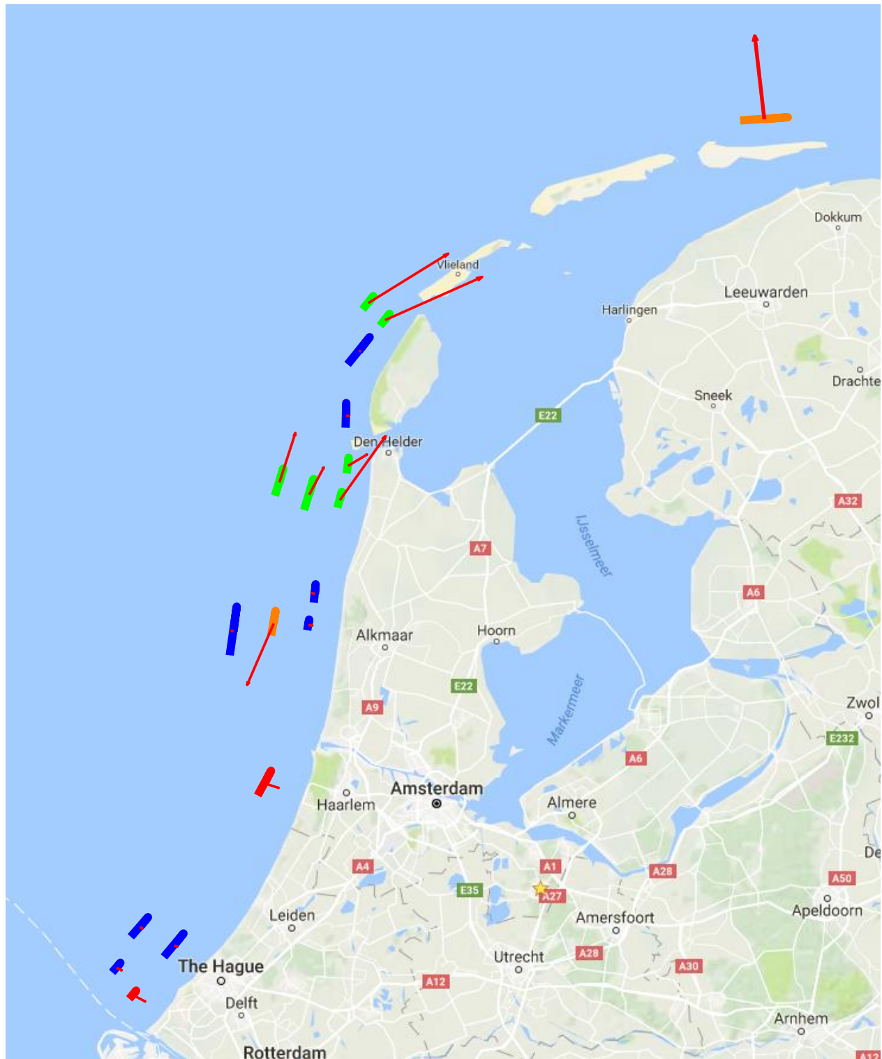
Figure 48: Visual migration of the shoreface nourishments along the Dutch coast. In this figure, the shoreface nourishments from the selection are shown with their migration given by the red arrow and the colour based on the cluster. When two or more shoreface nourishments are executed at the same location, the first one executed in time is the one closest to the coast. The second one is represented by the next one in row and so on. I.e. the shoreface nourishments are alongshore on the exact location, but cross-shore they are based on their execution phase and not the cross-shore distance to the coast. (Source of map: google.com)
