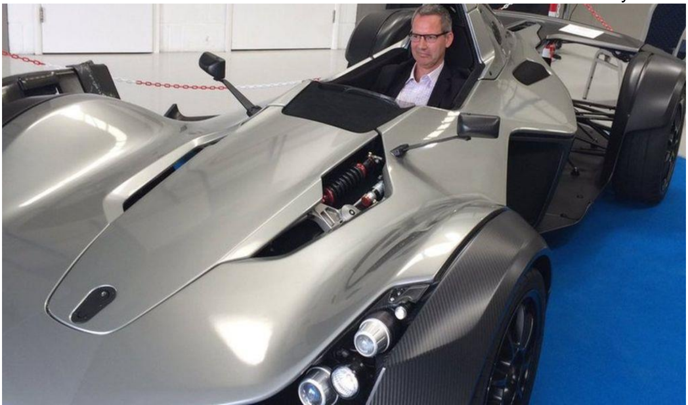
Briggs Automotive Company (2016): single-seater Mono sports car using graphene-enhanced resin in bodywork
