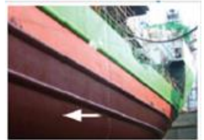
Ship hull coated with antifouling CNT paint (2008)
