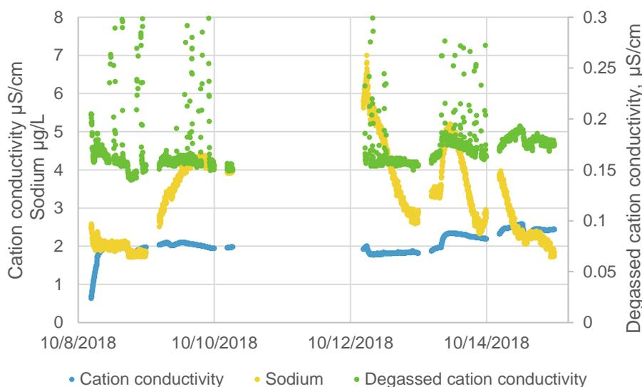
**Figure 13.** Online measurement of the cation conductivity, degassed cation conductivity and sodium during the second run in the RO permeate
