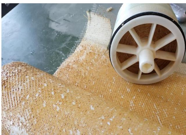
**Figure 17.** Visual inspection of the inlet cap and beginning of the feed channel
