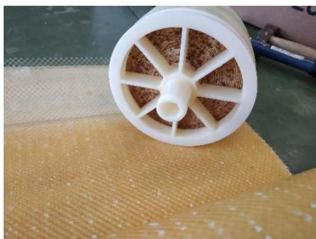
**Figure 18.** Visual inspection of the outlet cap and end of the feed channel
