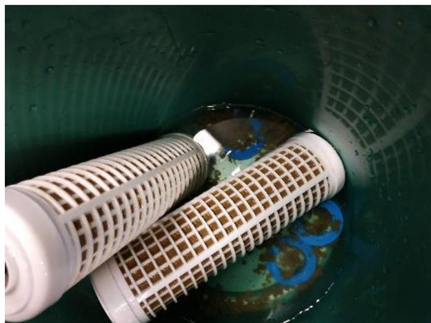
**Figure 16.** Fouling on the cartridge filters caused by F200
