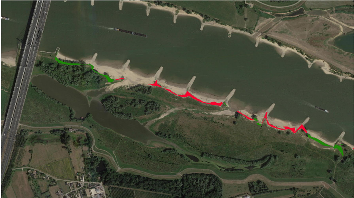
Figure 3.11 Changes in the vegetation pattern on the bank (photo 2019): red are the areas where the vegetation has disappeared, green where it has expanded.
