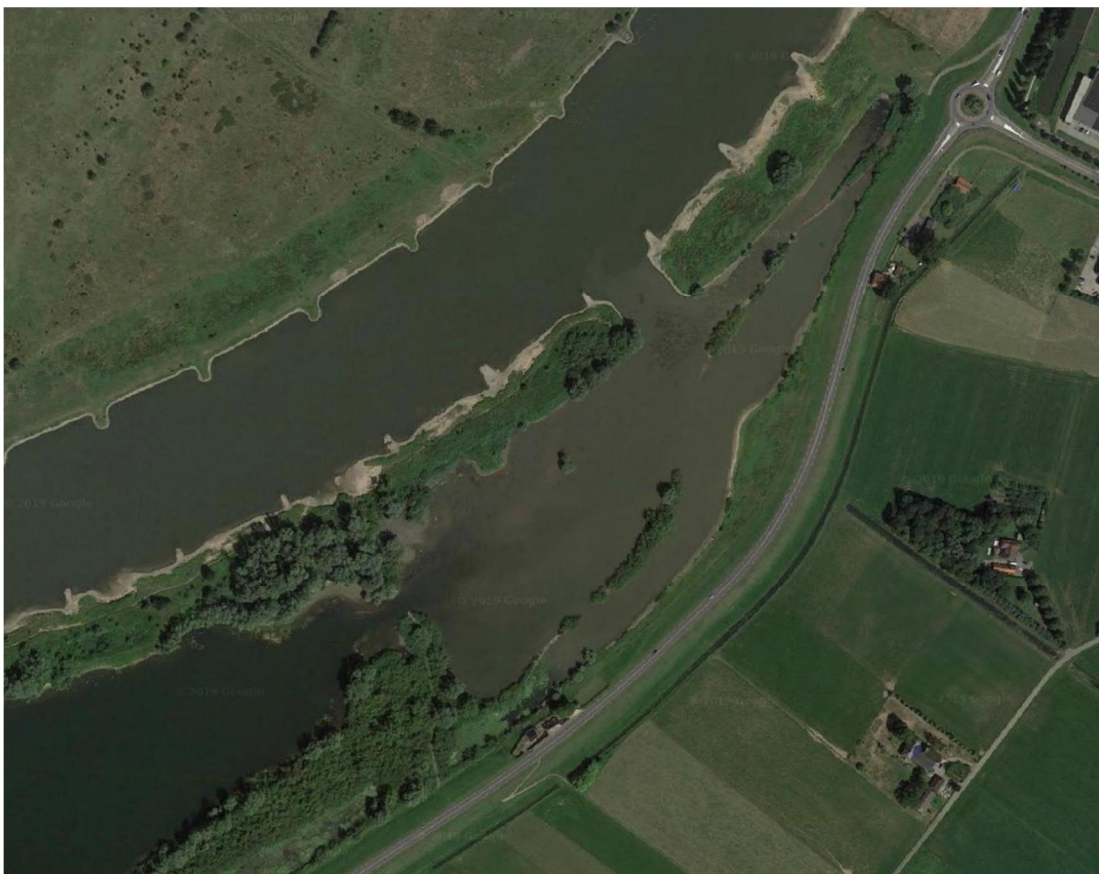
Figure 3.77 The northern lake is shallow and silt quickly swirls here. Part of this silt is then carried by outflowing water to the IJssel where a small plume is visible.
