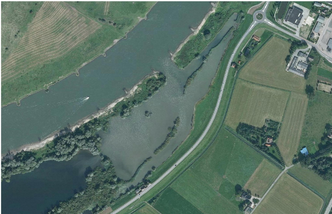
Figure 3.76 Turbid water from the IJssel flows into the channel system through the inlet, but the silt then sinks into the first deep pool on the left of the photo.
