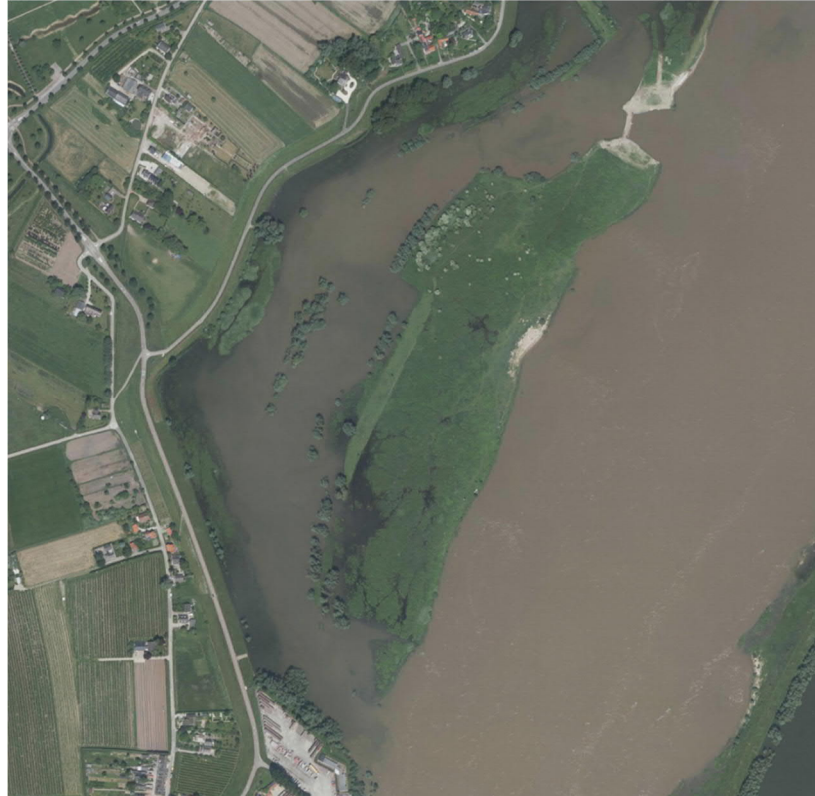
Figure 3.22 Photo with a slightly increased river discharge (Upper Rhine discharge approx. 3,500 m 3 / s). The water in the Waal contains more floating sludge that also flows into the secondary channel via the inlet. On the way through the secondary channel, this sediment partly settles and the water becomes clearer before it leaves the channel again.
