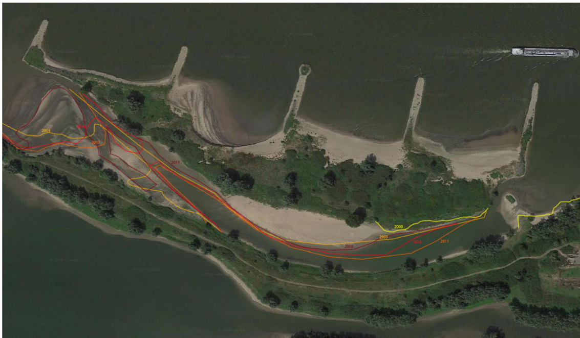
Figure 3.39 Changes in the contours of the sandbars in the secondary channel at low tide (2003, 2011, 2014 and 2019)
