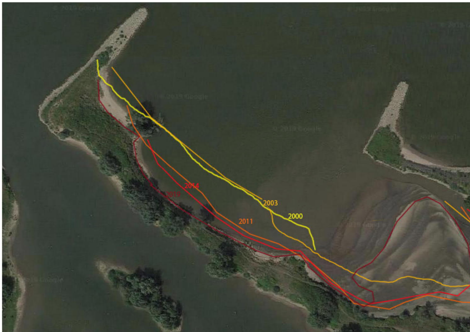
Figure 3.41 Contours of the bank in the outflow of the northwestern side channel over the period 2000 to 2019.
