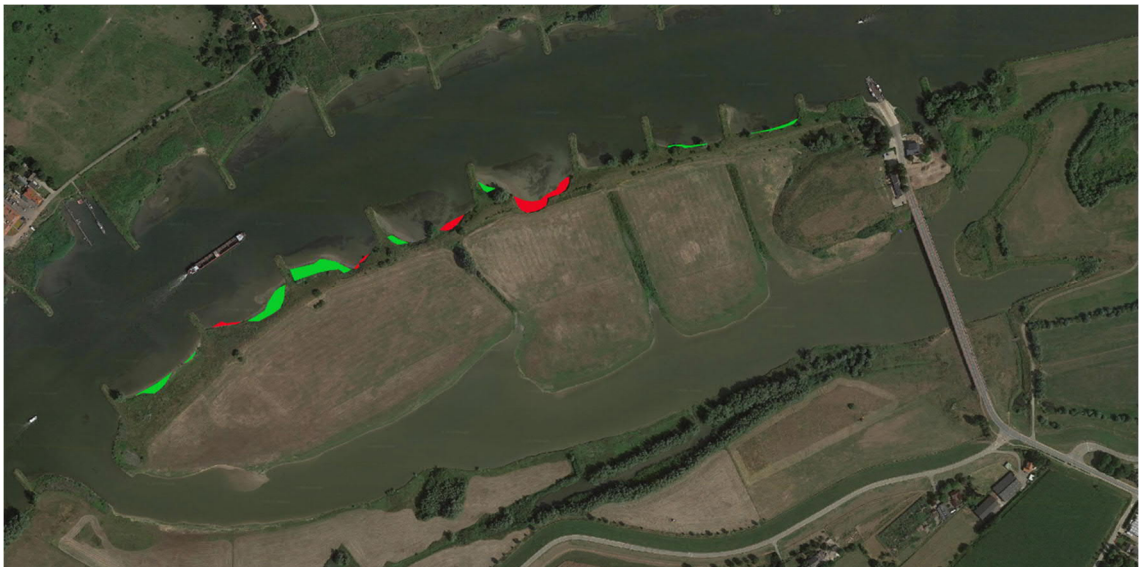
Figure 3.56 Changes in the bank line of the groyne sections between 2011 and 2019. In red the locations where the vegetation has disappeared and in green the locations that are now vegetated where previously there was open sand or water.
