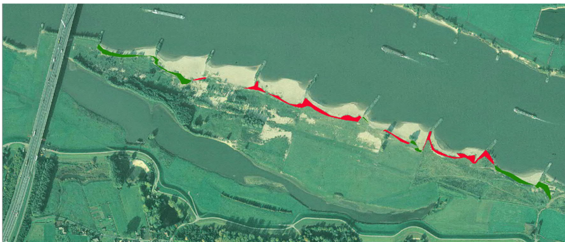
Figure 3.10 Changes in the vegetation pattern on the bank (photo 2007): red are the areas where the vegetation has disappeared, green where it has expanded.
