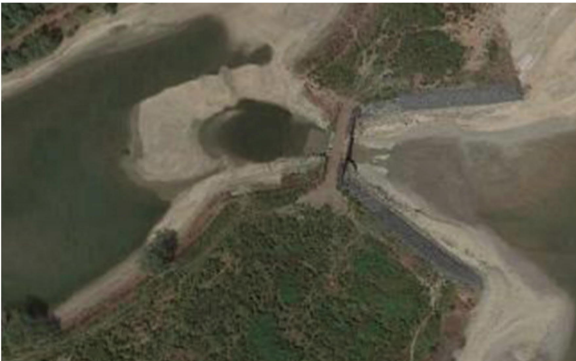
Figure 3.17 Erosion pit and annular sandbank immediately after the inlet of the flowing secondary channel. Photo taken during low water period in 2018.
