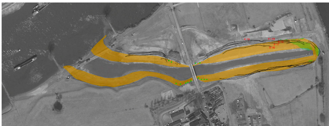
Figure 3.60 Contours of the eroding bank (black lines) with the month and year in red. The orange area is the gently sloping slope as-built. The outer edge of the orange surface is the insertion line and the inner edge is the edge of the flat bottom. The green areas are areas that have become overgrown in 2019 and have been sufficiently raised for this.
