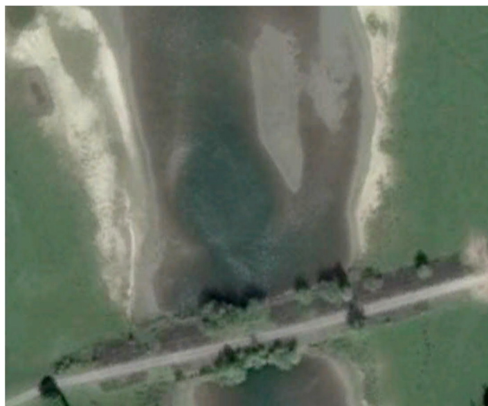
Figure 3.82 Erosion pit and sandbar immediately after the inlet works of the Vreugderijkerwaard (photo 2014)
