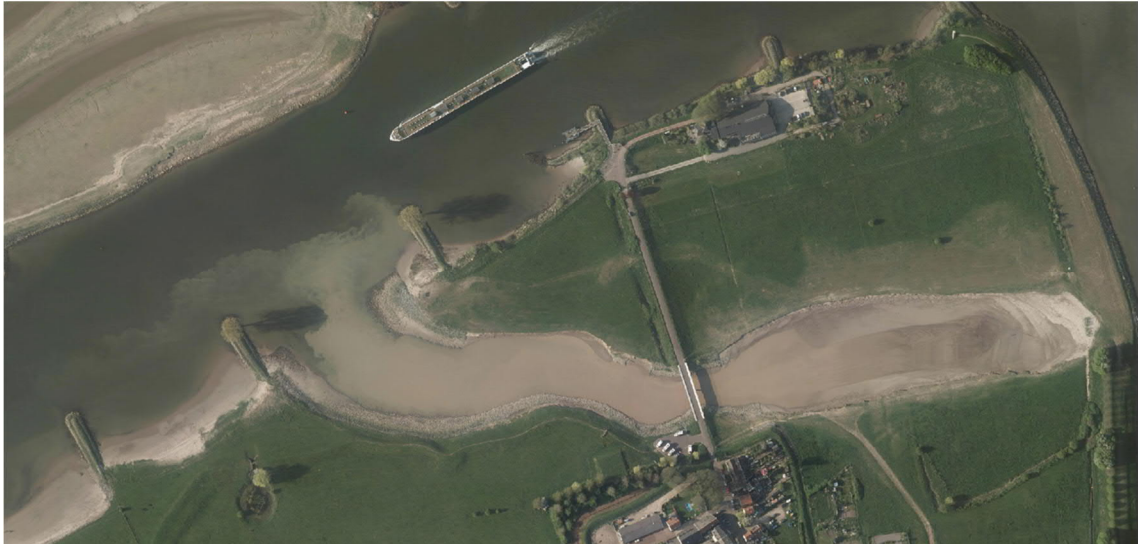
Figure 3.62 The channel is always filled with turbid water. During low tide the outgoing water flow carries some of the sediment into the river.
