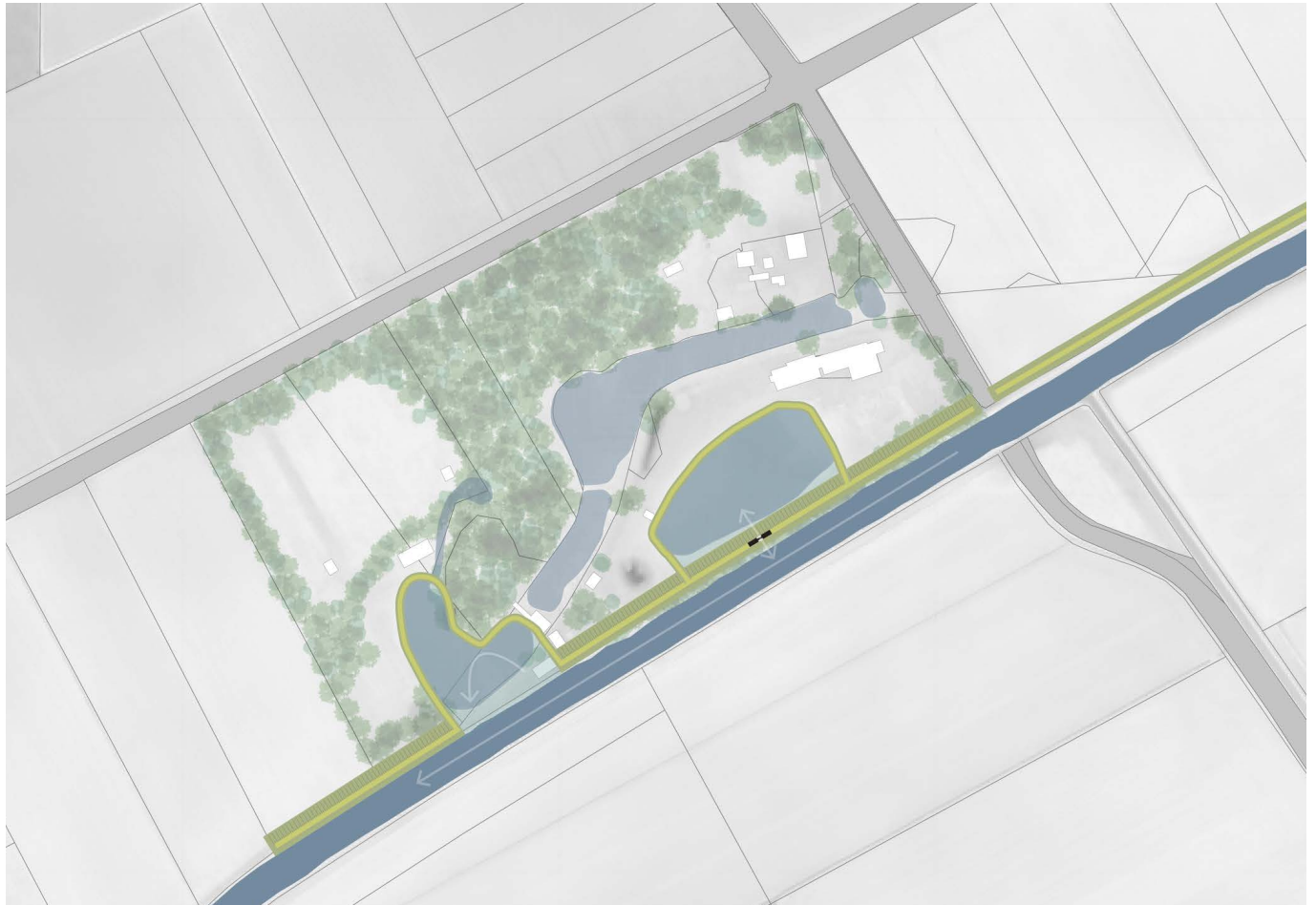
Widened dike slope combined with buffer basin
