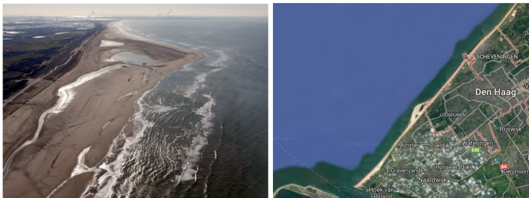
Figure 1: Sand engine at the coast of Delfland (from: M.D. Taal et al, 2016) and its position between The Hague and Rotterdam.
