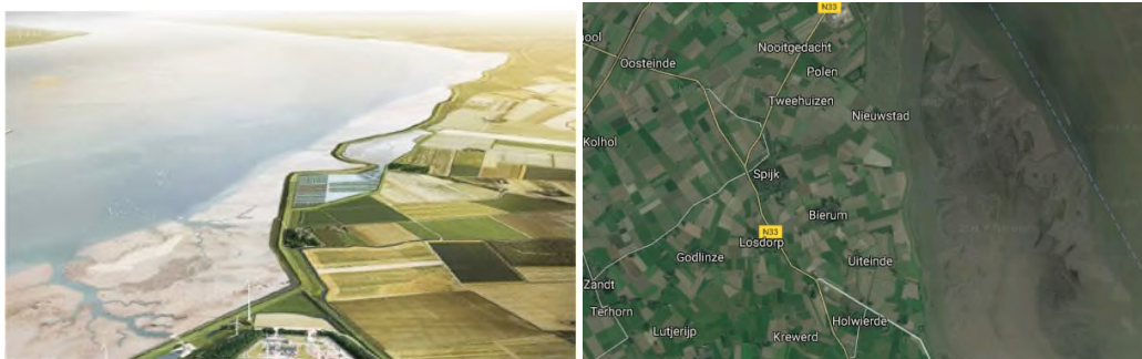
Figure 1: Overview of both sections with a double dike. The nearest section will be used as a clay factory/nature area and the second one for brackish agriculture. The area is situated north and south of Nieuwstad.
