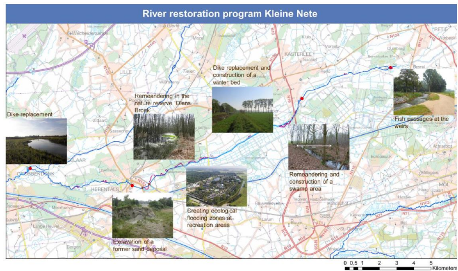
Figure 12 Project components of river restoration program Kline Nete (source: Flanders Environment Agency)
