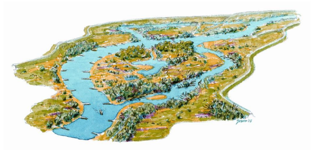
Figure 13 Secondary channel next to a main channel with groynes (Geerling & van Kouwen, 2010)
