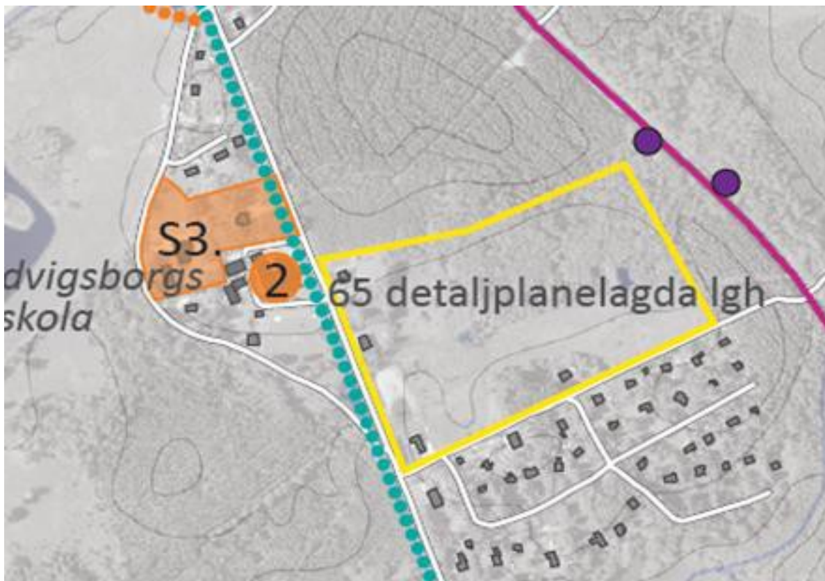
Figure 1. Cut-out from a comprehensive plan. The yellow marking is showing an adopted zoning plan with an area containing 65 planned apartments.
