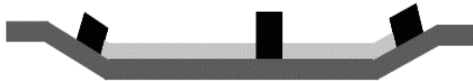
Step 2: Pre-forming the flexible foil circuit
