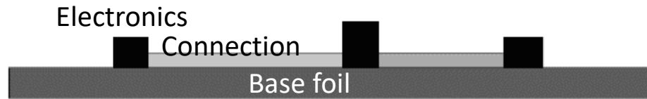
Step 1: Printing electronics on a flat foil to form the circuit
