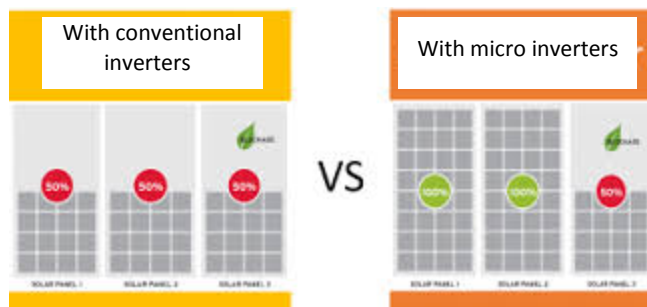
Pic. 2.24: Shading impact at conventional and micro inverter
