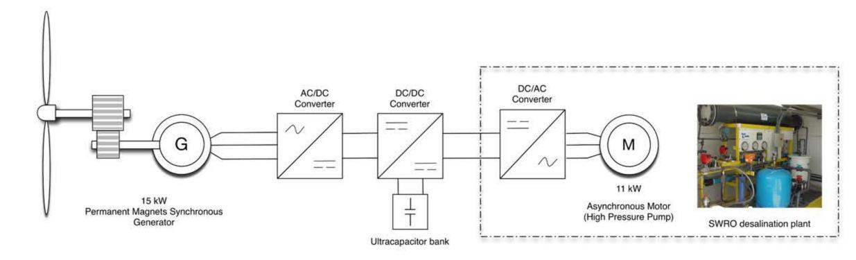
Fig. 1. General configuration of the wind energy based microgrid designed to desalinate seawater.
