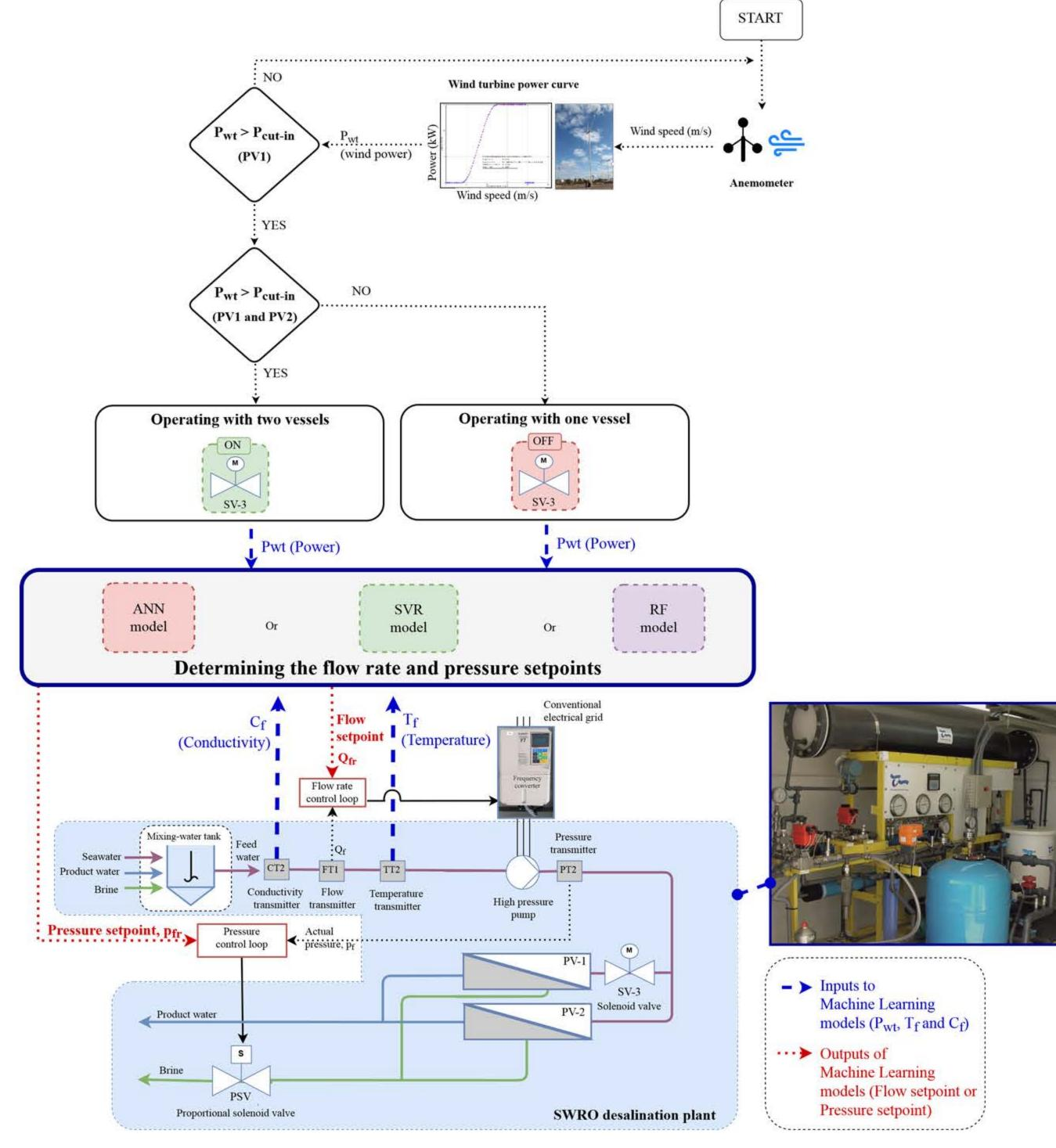
Fig. 2. Layout of the SWRO desalination plant prototype and control system.
