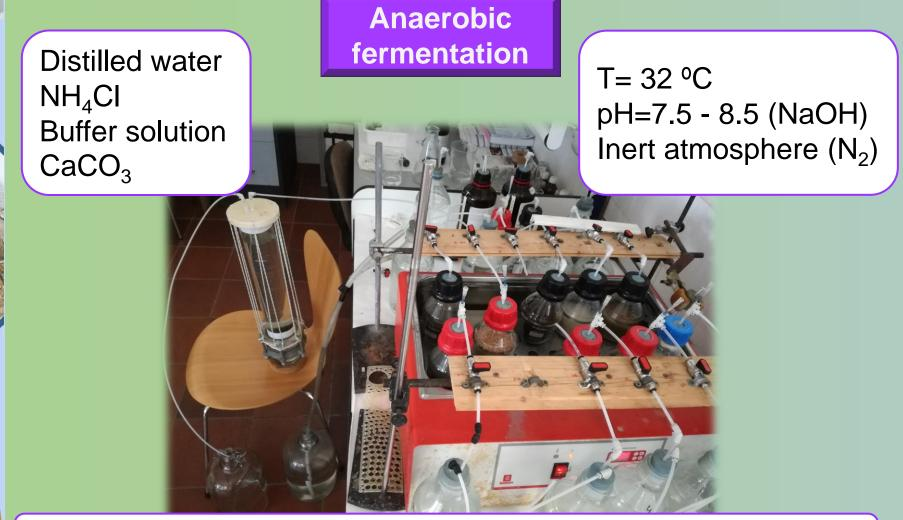
Biogas production finished → pH reduction → reactivated with NaOH
