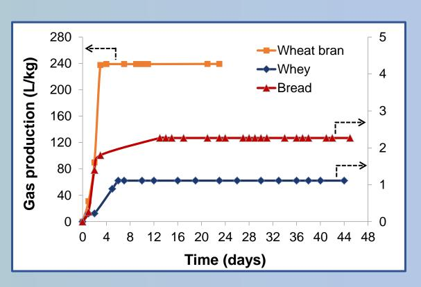
\* The highest gas production without reactivation is obtained for the wheat bran, 240 L/kg in 4 days.
