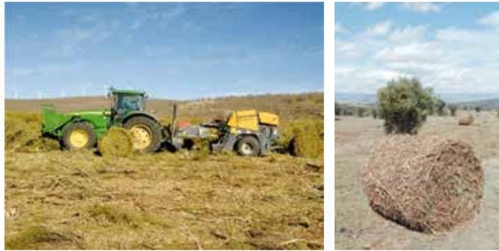
Figure 1. Harvester-baler system and round bale
