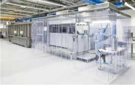
*Inline tool for the cost-efficient epitaxy of 150 µm thick and highly pure Si layers.*
