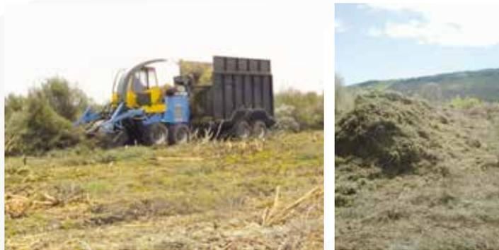
Figure 2. Harvester-mulcher system and collected biomass
