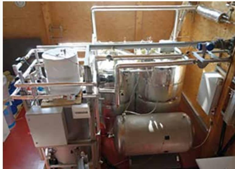
solar heat is used to drive the water vapour out of the zeolite and the released vapour is condensed at the evaporator/condenser heat exchanger again and the heat of condensation is transferred to the low temperature heat sink in this case. The storage system is under vacuum and therefore a low temperature level is sufficient to evaporate the water.
