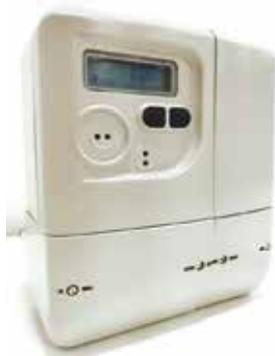
Smart Low-Cost advanced meter prototype
