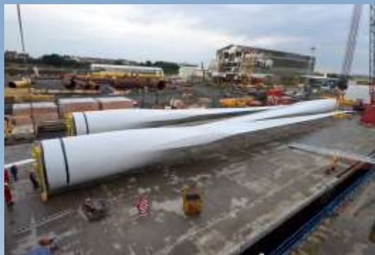
Samsung 7MW turbine – Blade unloading
